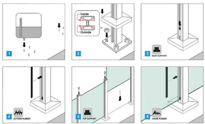
Tip: The top & base supports are universal, and the side with rubber is slways next to glass - when placed as a base support, the rubber is upward, while as a top support, the rubber is facing down.
