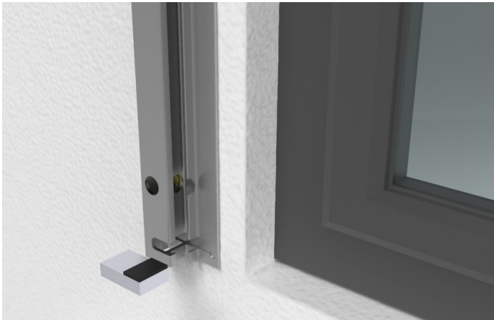
Aluminium support block ensures reliable glass retention
